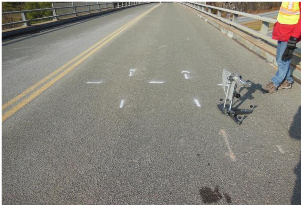
Figure 4. Layout of skid testing locations, wheelpath (right) and non-wheelpath (left). The British pendulum tester can also be seen.
