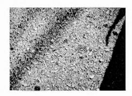
Glasphalt Pavement (front) / Standard Mix (back)
