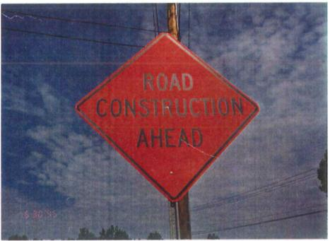
**FOLLOW UP:** The material should continue to be used on signs relating to construction. Additional data should be collected, and further evaluated to determine the overall effectiveness of the Fluorescent Diamond Grade material.
