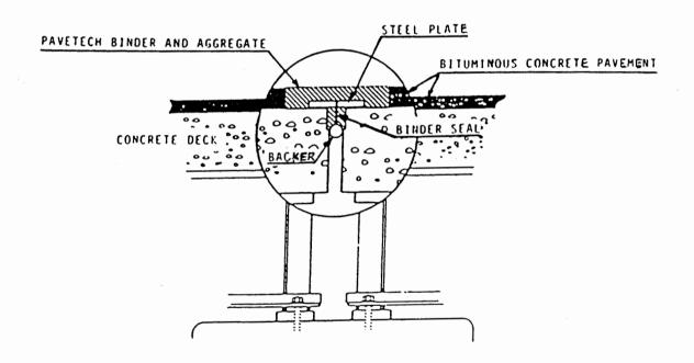
TYPICAL PAVETECH CROSS SECTION
