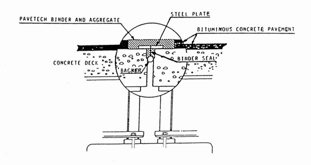
TYPICAL PAVETECH CROSS SECTION
