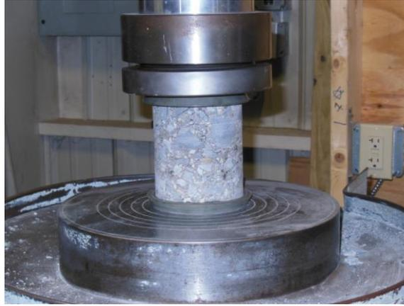
**Figure 7 Compression test on a core.**
