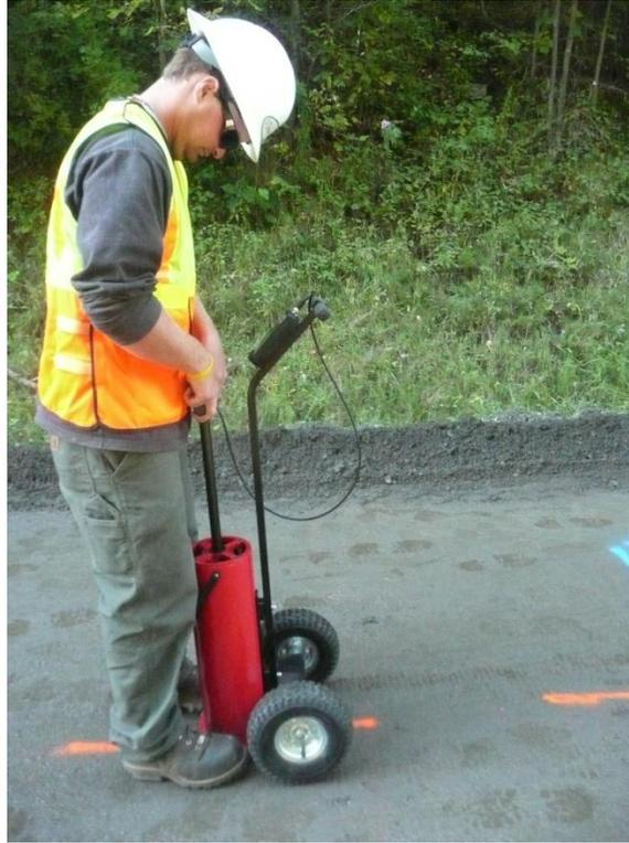
**Figure 3 Clegg Impact Soil Tester (CIST) being used to collect data on a project.**
