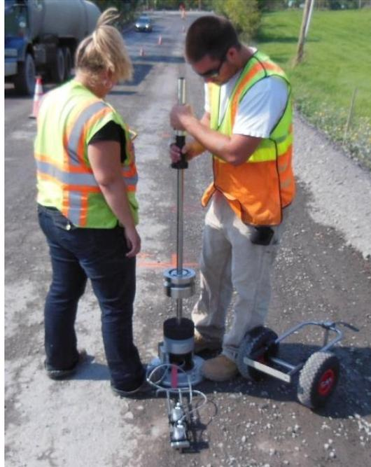
**Figure 4 Light Weight Deflectometer (LWD) being used to collect data on a project.**
