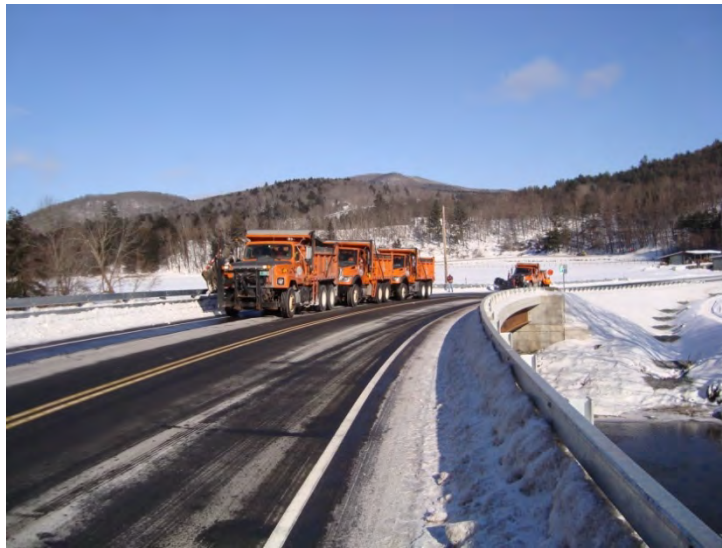
Figure 5-17: Stockbridge Bridge Load Testing
