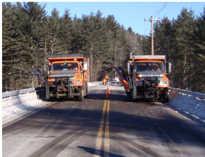
Figure 5-4: Middlesex Load Testing (Transverse Arrangement of Trucks)
