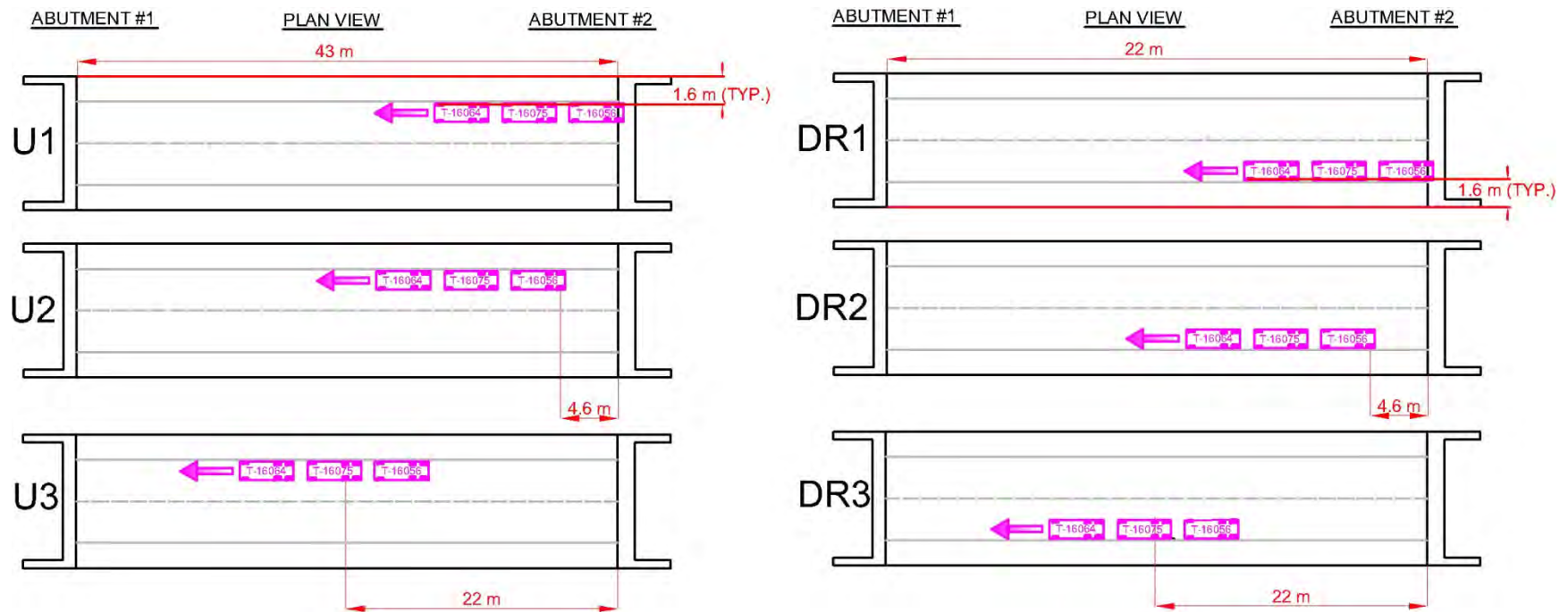
Figure 5-7: Middlesex Load Testing Truck Locations (Upstream Lane – Forward and Downstream – Reverse)
