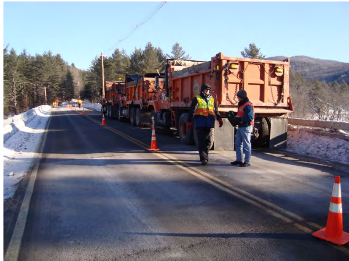
Figure 5-2: Middlesex Load Testing (Longitudinal Arrangement of Trucks)
