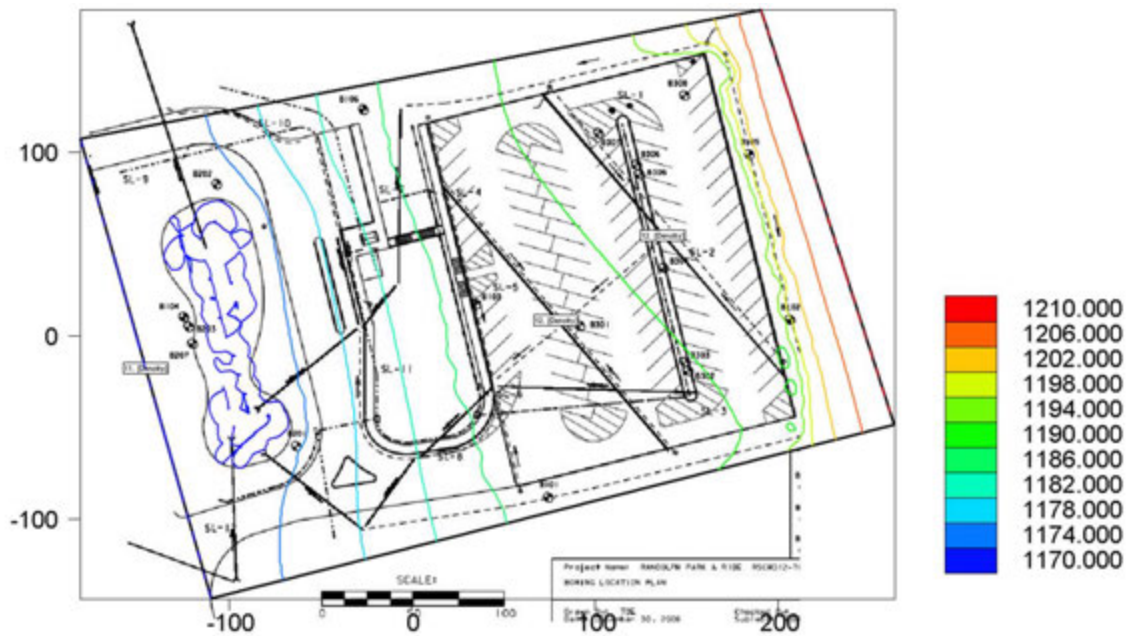
Figure 4.8: Top Layer (3rd) - Steady state conditions for total head (units in ft).
