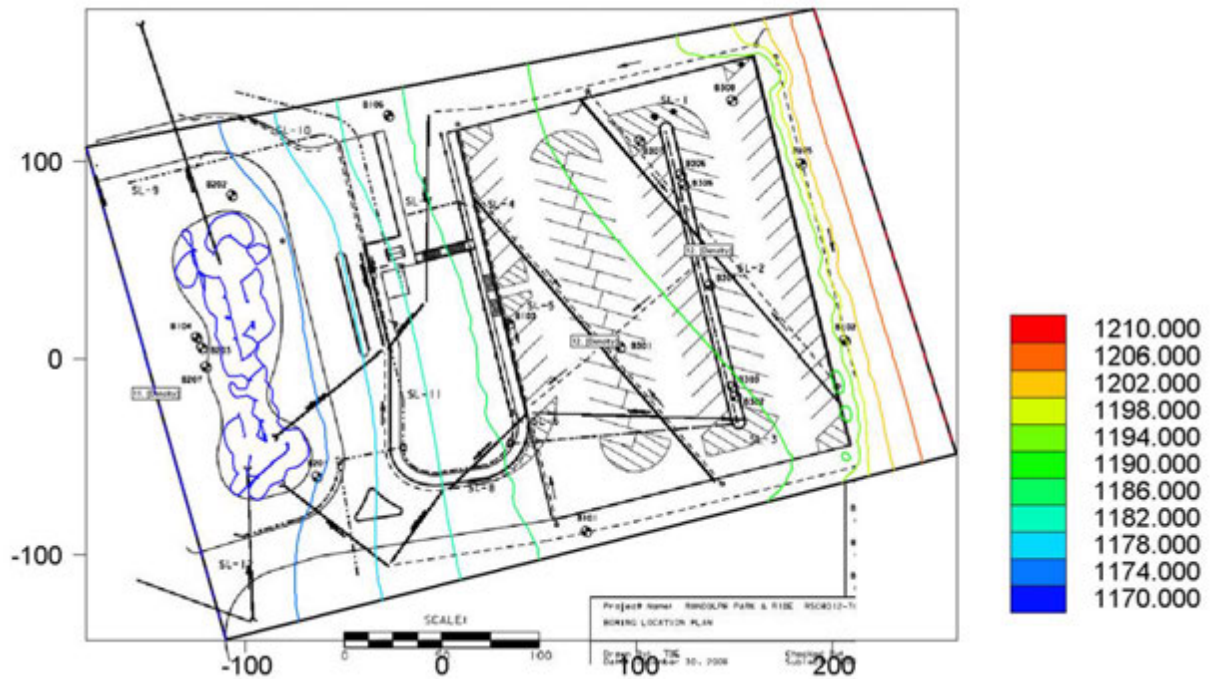
Figure 4.10: Top Layer (3rd) - Total head (units in ft) 10 days after the rainfall event.
