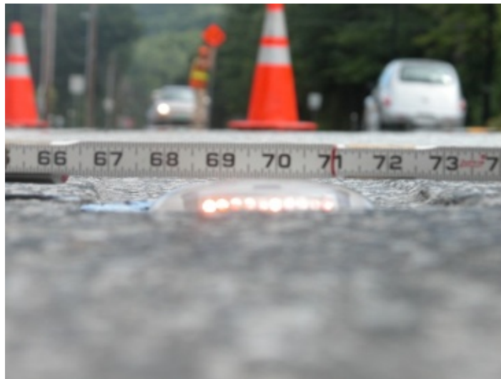
FIGURE 7 Domes are slightly above road surface.
