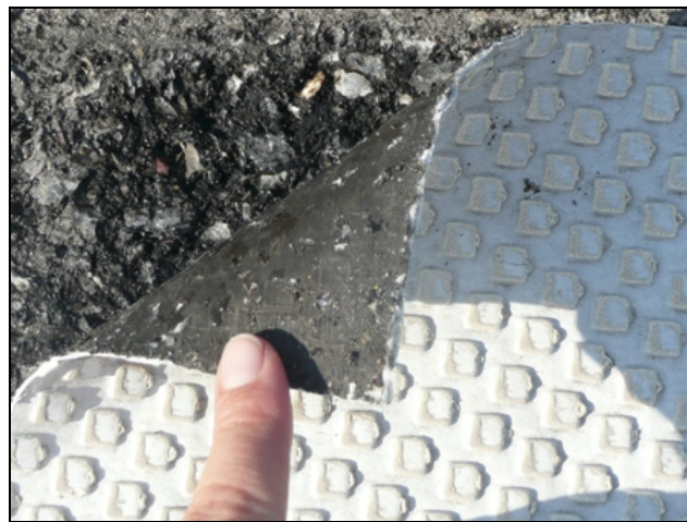
Figure 2. Ease of pull-up of the installed 3M tape.
