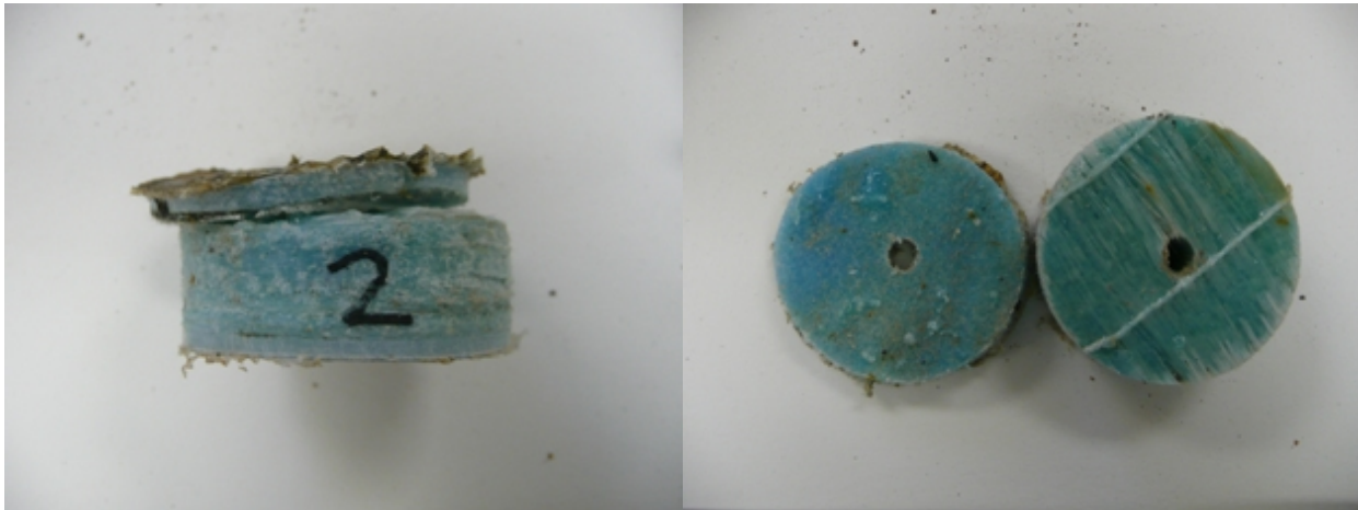
Figure 5. Photographs of sample 2, showing separated layers.
