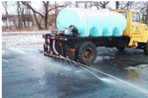
District 5's Tanker and Spray-bar system
