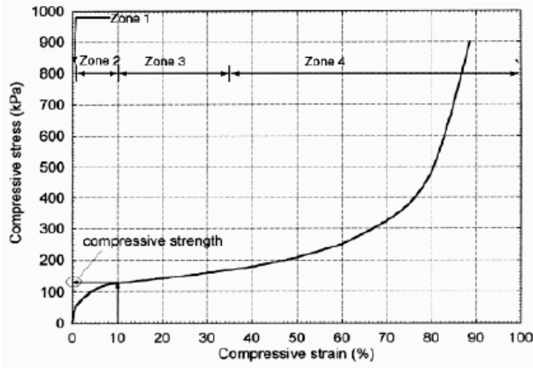
**Figure 2.1. Typical Stress-Strain Response of 21 kg/m<sup>3</sup> EPS Geofoam at 10% strain per minute (from Stark et. al. 2004).**
