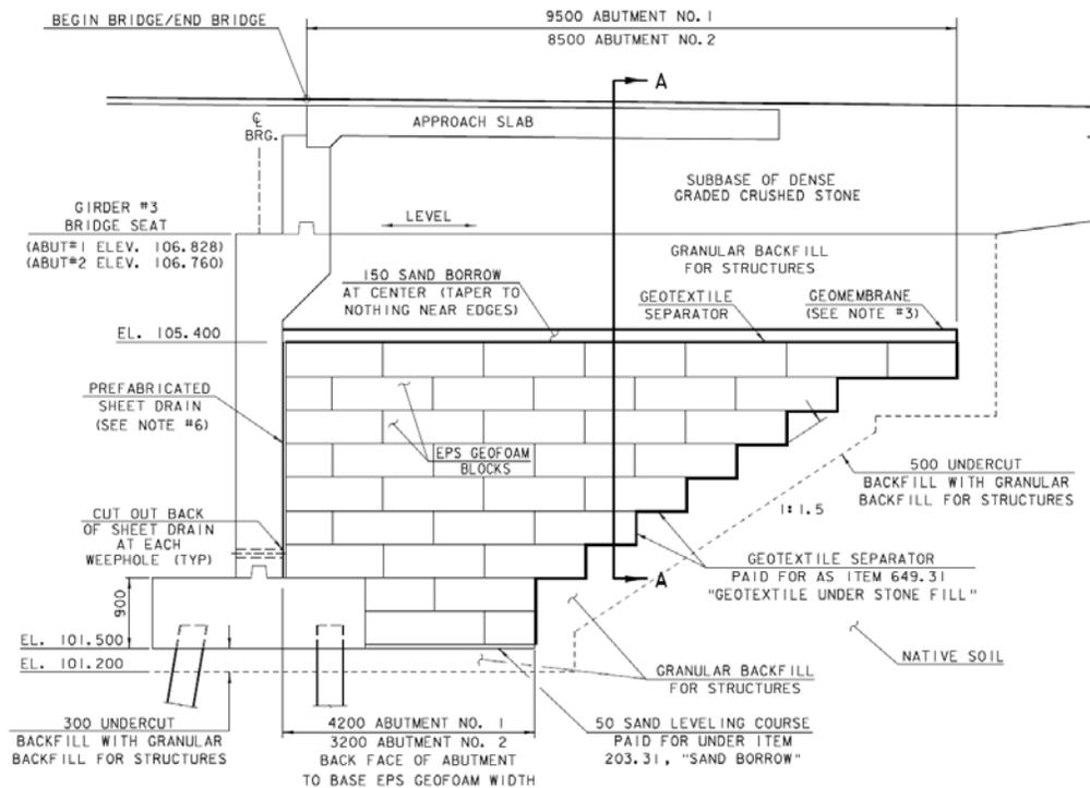
**Figure 3.6 Typical Abutment Cross Section (Facing Perpendicular to Centerline).**
