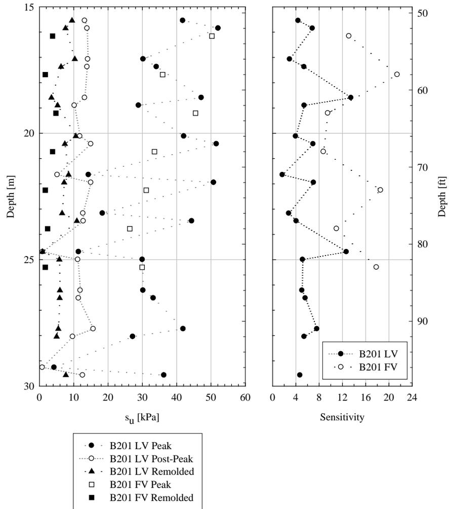
**Figure 4.5 Variation in Undrained Shear Strength with Depth.**
