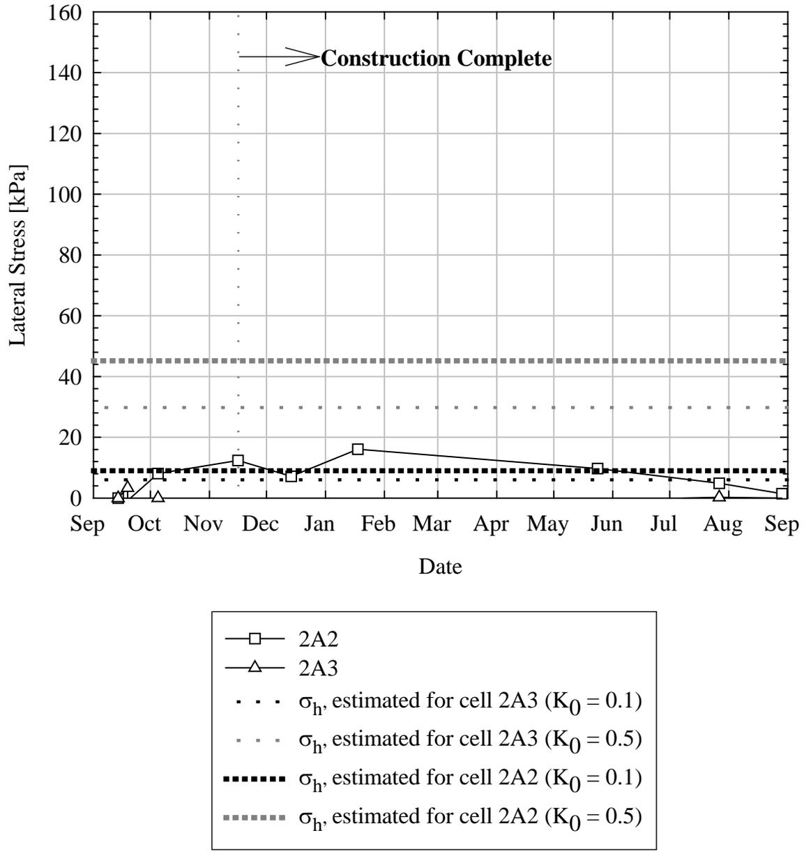
**Figure 6.24 Estimated and Measured Lateral Pressures at Abutment 2 versus Time for Case IV Loading.**
