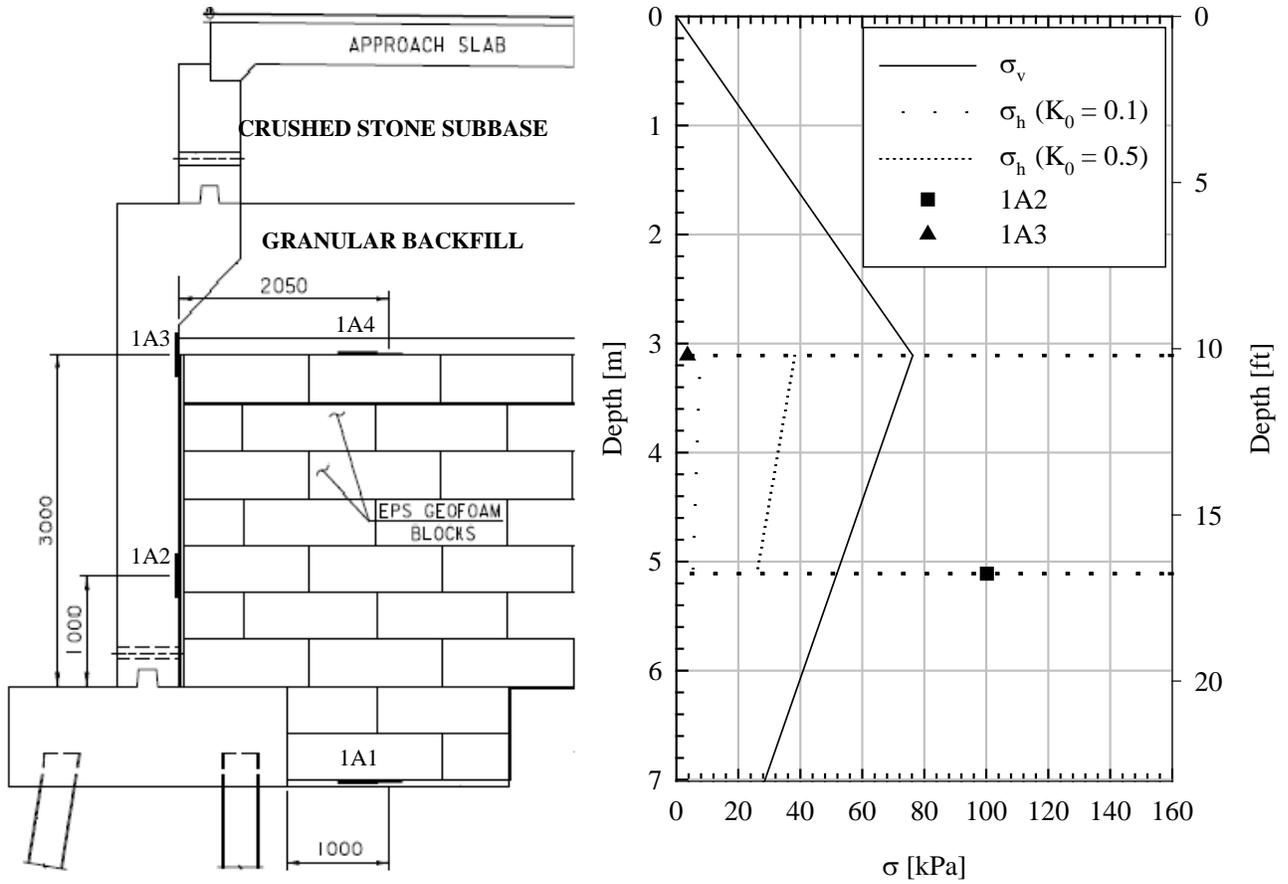
**Figure 6.21 Estimated and Measured Vertical and Lateral Pressures at Abutment 1 for Case IV Loading.**
