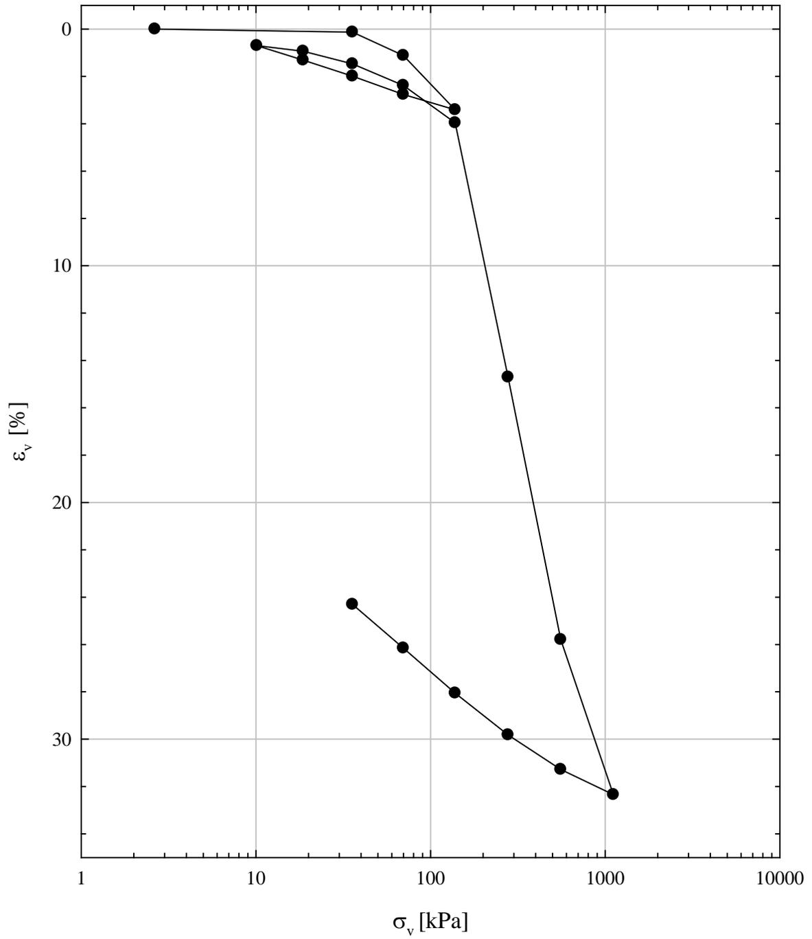
**Figure A.1 Incremental Load Consolidation Test Results for Borehole B-201, 15.5 m (51.0 ft).**
