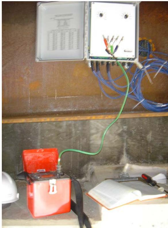
**Figure 5.6. Central Breaker Box and Geokon GK-403 Vibrating Wire Readout Box.**
