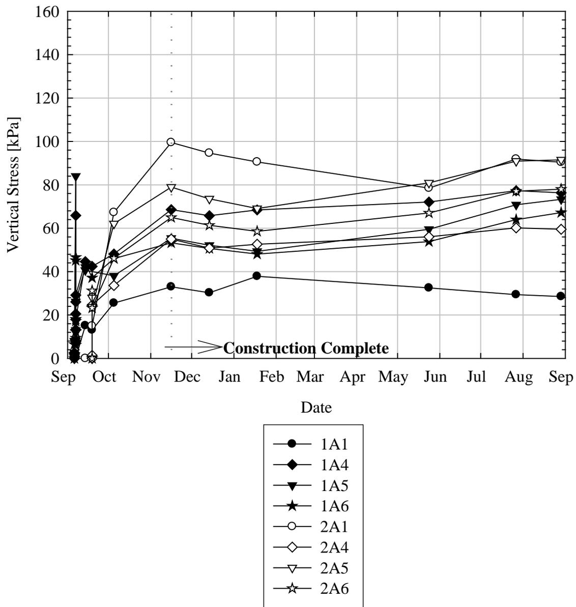
Figure 6.7 Vertical Pressures Measured at Abutments 1 and 2 versus Time.
