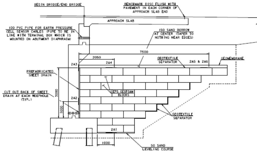
**Figure 5.2 Earth Pressure Cell Locations (Abutment 2 Shown).**
