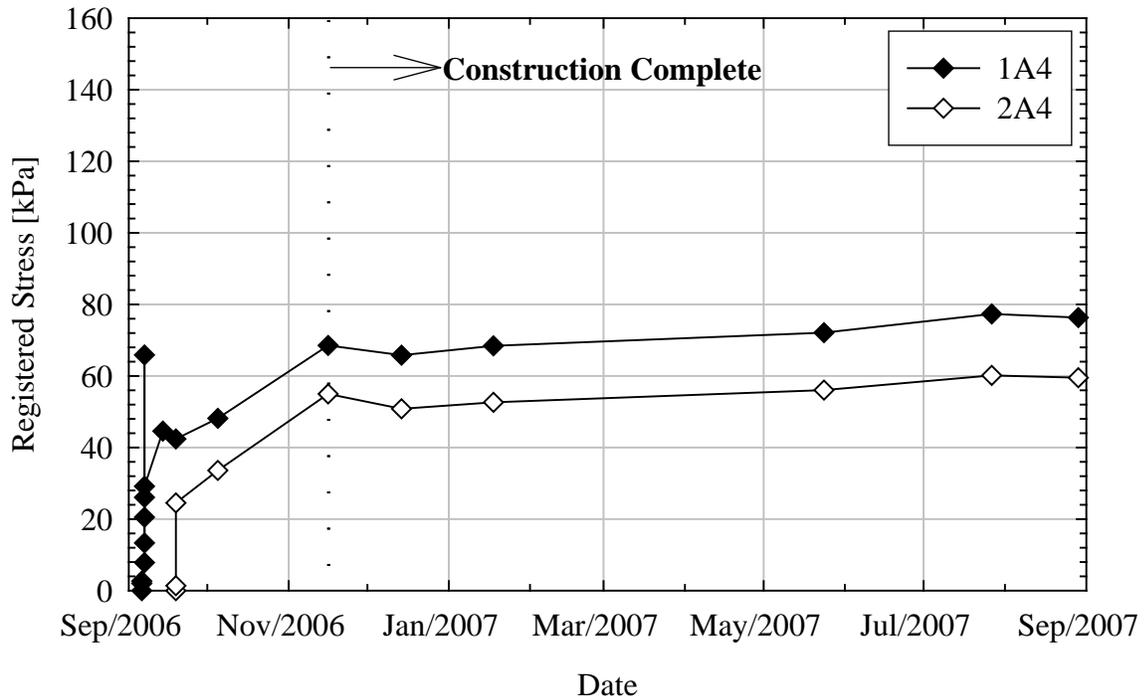
**Figure 6.4 Measured Vertical Earth Pressures versus Time for Transducers 1A4 and 2A4 (Top of GeoFoam Blocks, Centerline of Abutments).**
