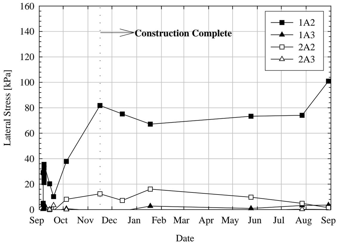
**Figure 6.8 Lateral Pressures Measured at Abutments 1 and 2 versus Time.**
