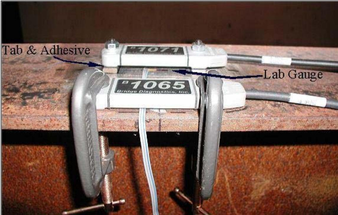
**Figure A.3: 2 BDI Gauges and Laboratory Gauge Attached to Top Flange**
