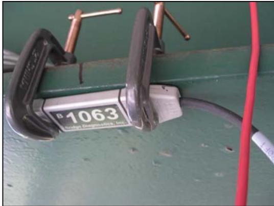
**a) Clamped Strain Gauge**
