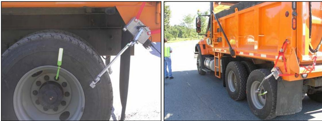
**Figure 4.3: Photographs of AutoClicker Attached to Load Vehicle**
