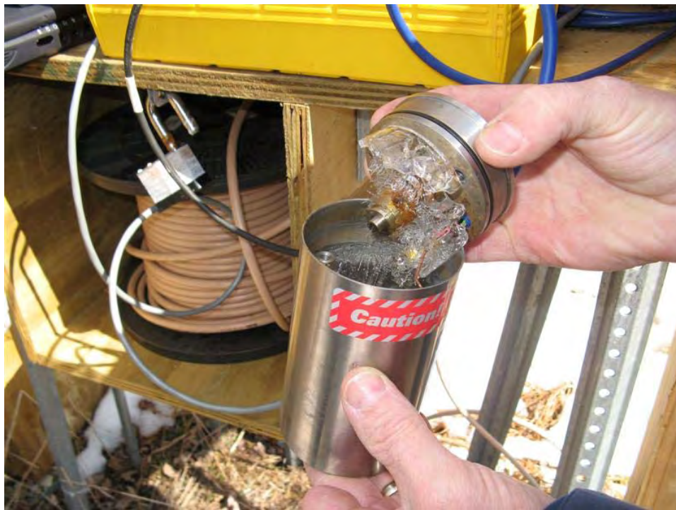
Figure 3.6 Ice damage inside the sealed barometer.
