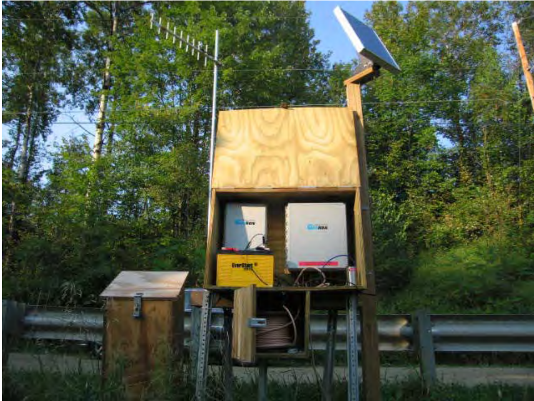
Figure 3.10 View of the data acquisition system when the protective box is open. The battery is in the front left, the multiplexer behind, and the datalogger to the right. The cell phone antenna is in the upper left and the solar panel in the upper right.
