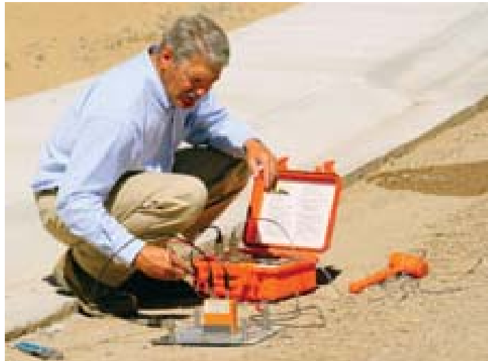
Figure 4: Typical EDG test set-up
