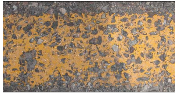
Figure 8 – Test Site 5 Yellow Edge Line May 30, 2007, Wear Rating = 5
