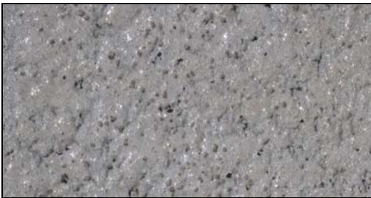
Figure 5 – Test Site 5 White Edge Line July 30, 2003, Wear Rating = 10
