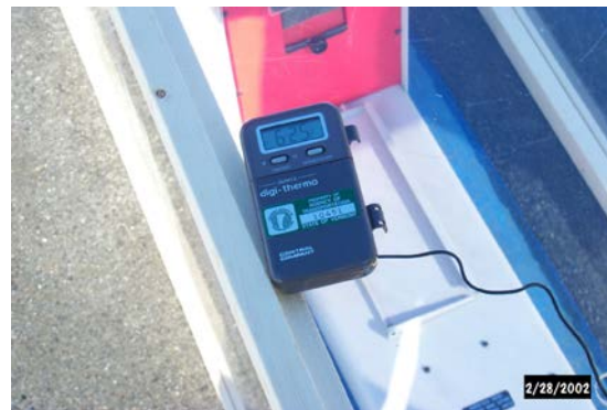
Figure 9. Temperature reading within Plexiglas™ box.
