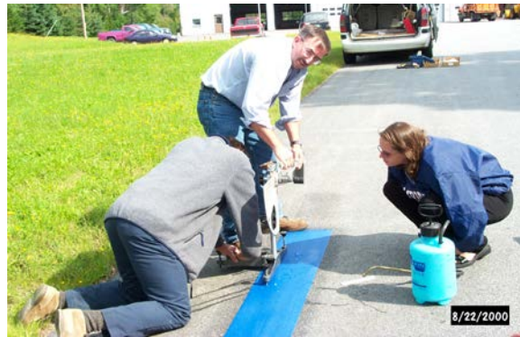
Figure 10. Skid test with British Pendulum Tester.
