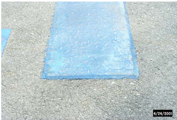
Figure 13. Test Strip A (west end) with feathered edge after eight months.
