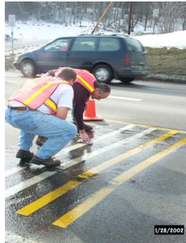
Figure 8. Drying markings on test deck. (Photo taken January, 2002)
