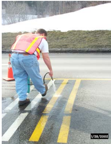
Figure 7. Cleaning markings on test deck. (Photo taken January, 2002)
