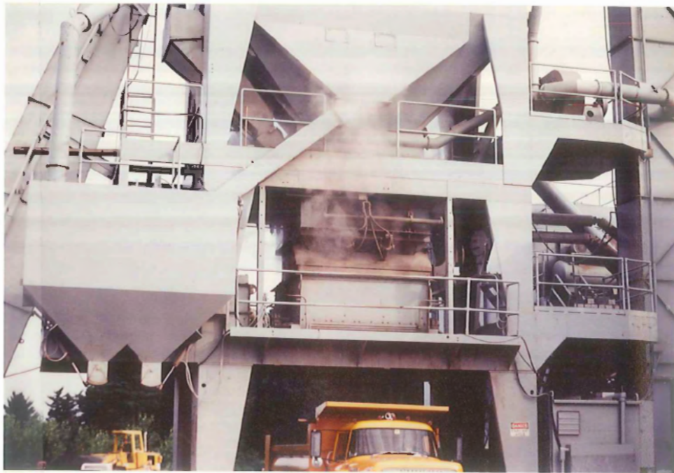
Figure 8 Normal Emissions At Pug Mill During Dry Mix Cycle
