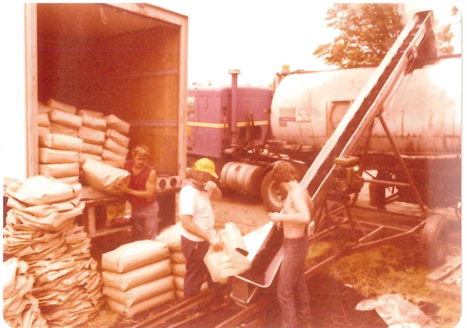
Introducing crumb rubber by means of a conveyor system
