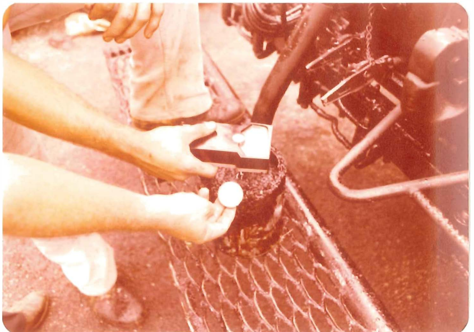
Measuring asphalt rubber viscosity following reaction period.
