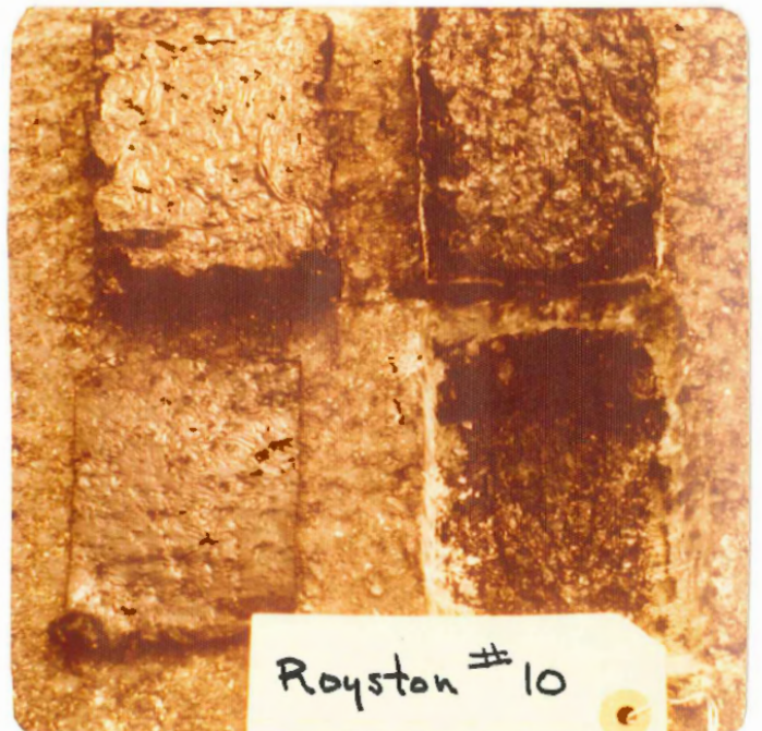
Removal of compacted pavement revealed no damage to the membrane
