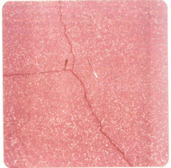
Cracks in Gussasphalt
