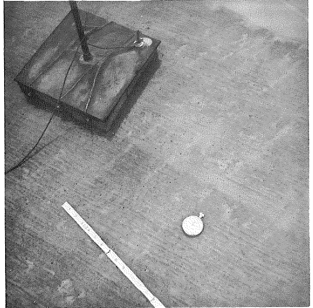
Electrical resistance readings averaged 41,500 ohms per square foot which indicates that some of the holes were open to the concrete.
