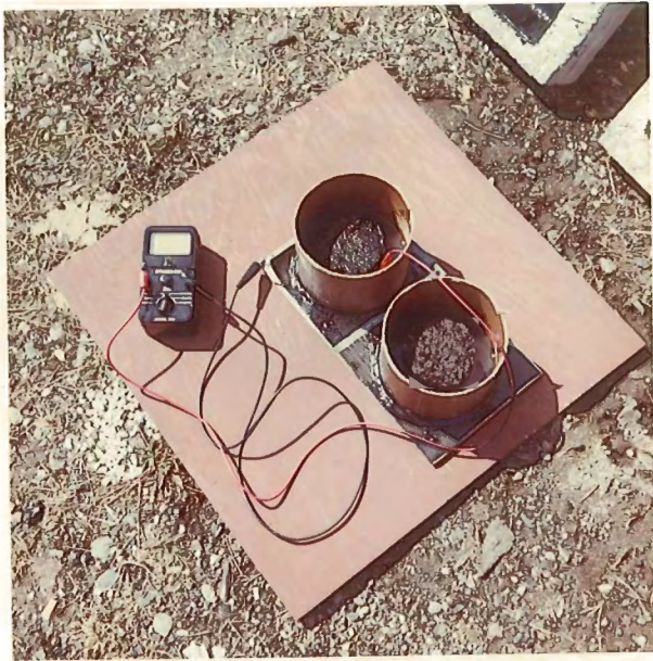
Puncture resistance of preformed sheet membranes being checked with an electrical resistance test
