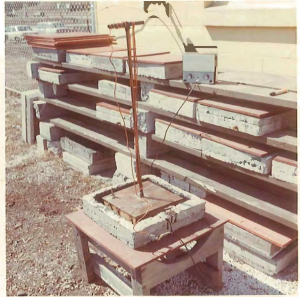
Laboratory and field applied membrane coatings are periodically checked for decreases in electrical resistance
