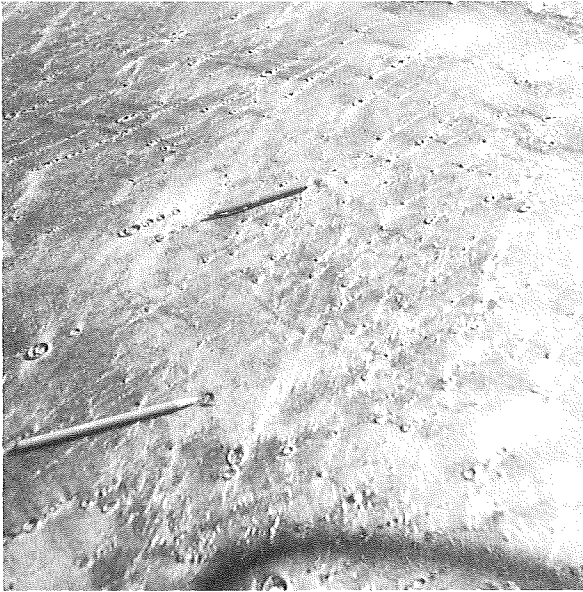
When air bubbles were broken open, little more than primer was detected on the concrete in many cases.
