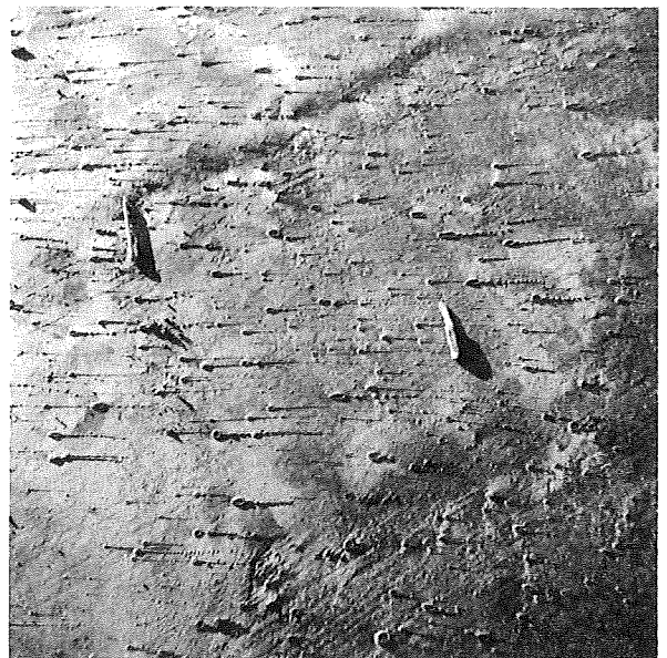
Air bubbles and craters in the cured membrane.
