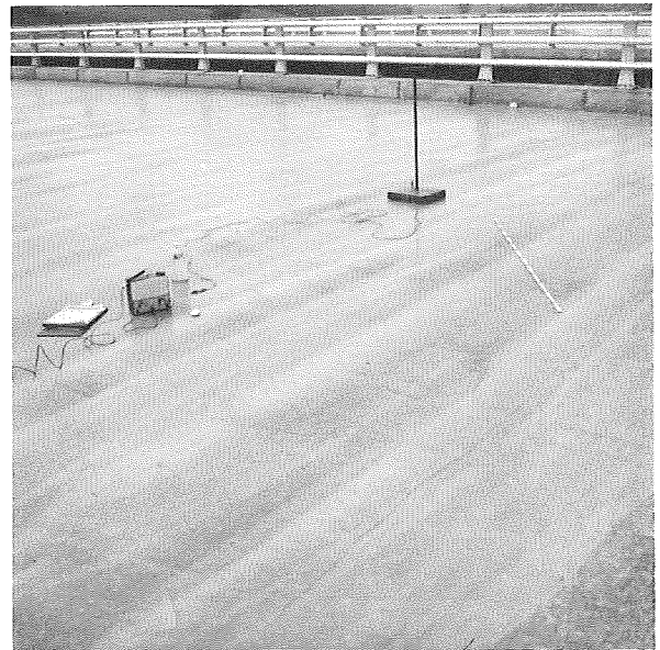
Testing with hydrochloric acid disclosed that the air bubbles and pinholes were not open to the concrete. Resistance readings were high, averaging 1.2 million.
