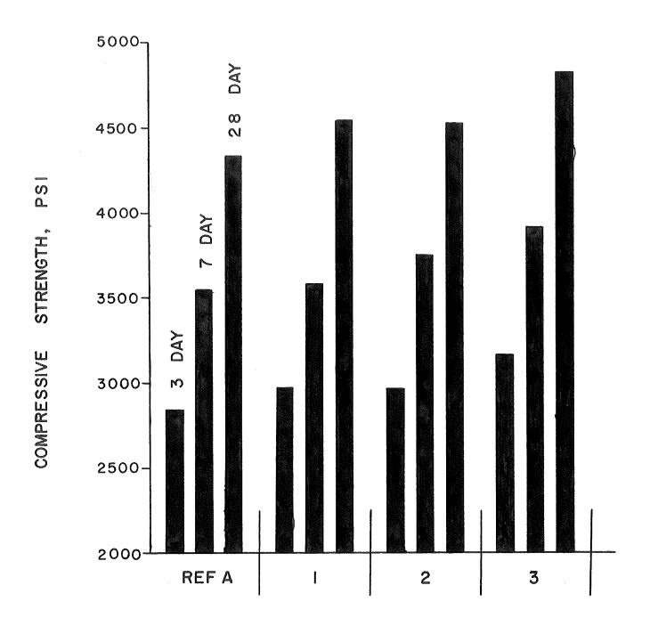
FIGURE IV-A COMPRESSIVE STRENGTH TESTS
