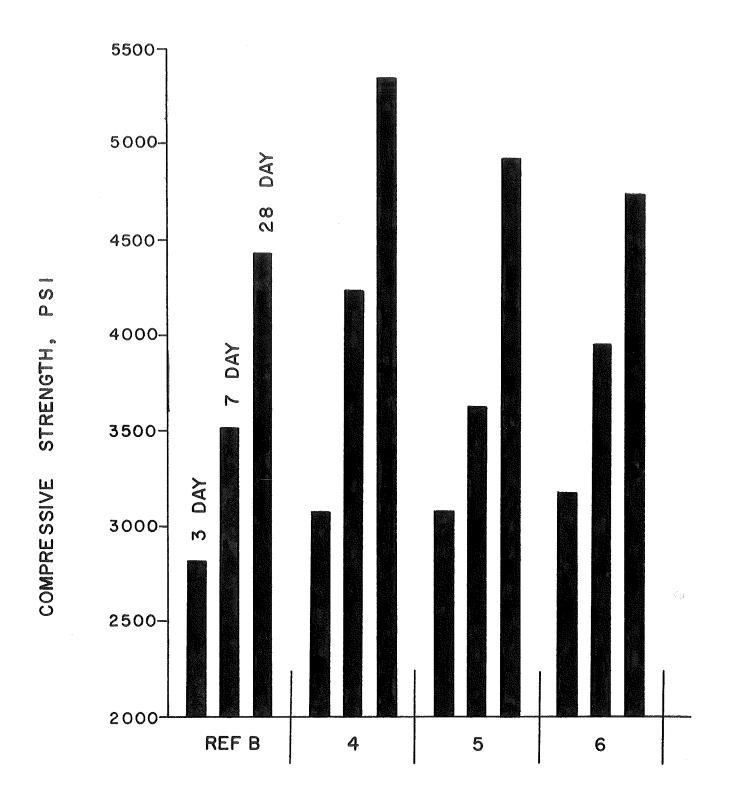
FIGURE IV-B COMPRESSIVE STRENGTH TESTS
