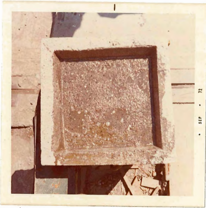
Air bubble clusters in first coat placed on concrete test slab
